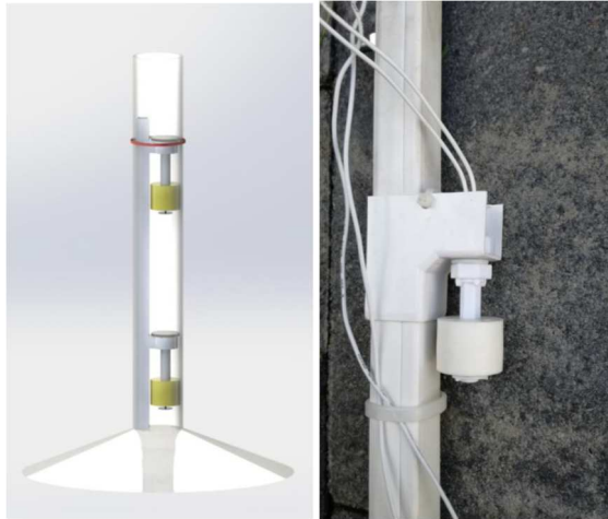
Figure 7 Float level reed sensors installation
