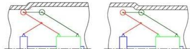
Figure 5 Changing the pipe diameter
