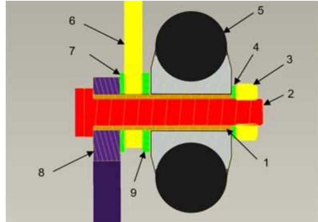
1 – sliding bearing; 2 – screw; 3 – nut; 4, 7, 9 – mat; 5 – idler wheel; 6 – connecting arm; 8 – arm
