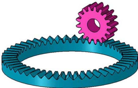
Figure 7 Face gearing model
