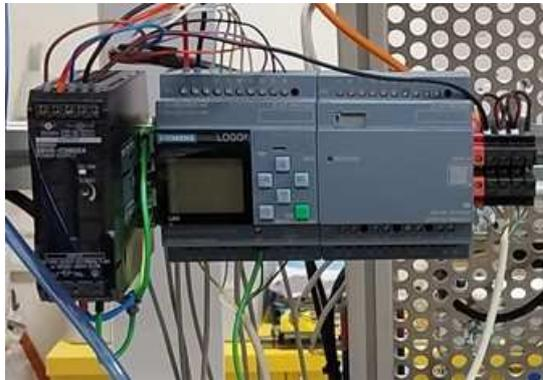
Figure 8 PLC control unit with expansion module in SIEMENS LOGO! v. 8.4 version
