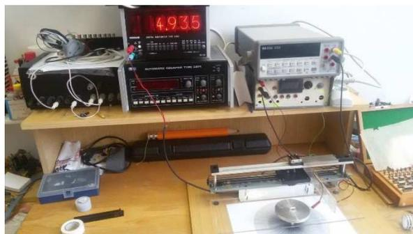
Figure 4 Experimental testing of the Hall-effect distance sensor
