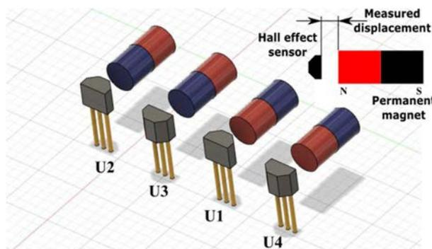
Figure 5 Sensor and permanent magnet arrangement options configurations
