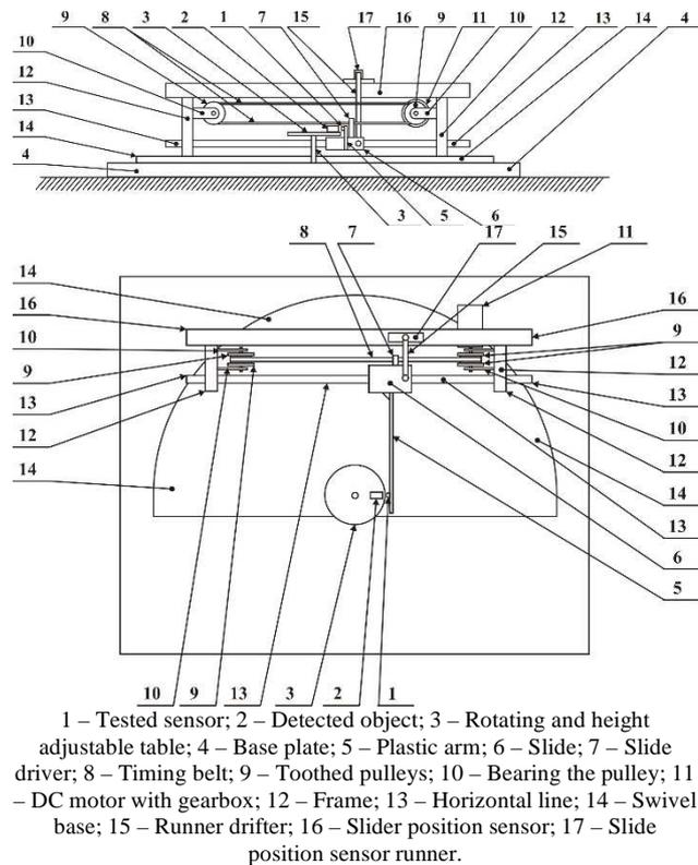
1 – Tested sensor; 2 – Detected object; 3 – Rotating and height adjustable table; 4 – Base plate; 5 – Plastic arm; 6 – Slide; 7 – Slide driver; 8 – Timing belt; 9 – Toothed pulleys; 10 – Bearing the pulley; 11 – DC motor with gearbox; 12 – Frame; 13 – Horizontal line; 14 – Swivel base; 15 – Runner driver; 16 – Slider position sensor; 17 – Slide position sensor runner.
