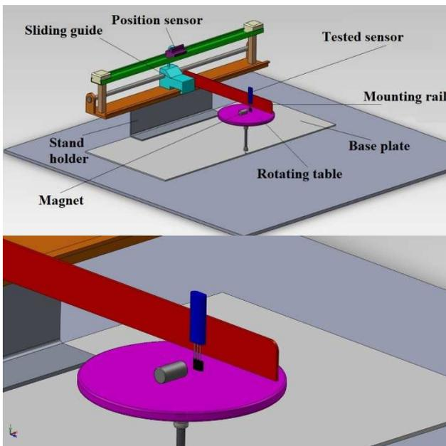
Figure 2 Length sensor tester concept
