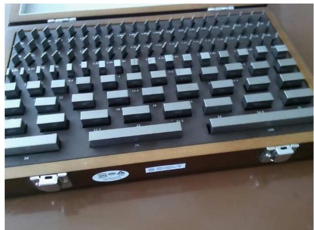
Figure 1 Set of parallel gauge blocks
