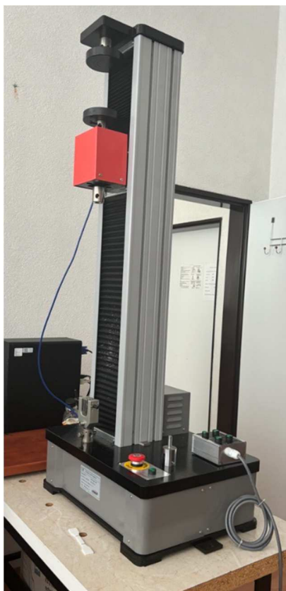
Figure 6 Universal testing machine designed for tensile and compression testing
