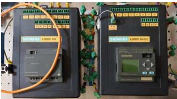
Figure 5 SIEMENS LOGO! PLC modified for use on a trainer
