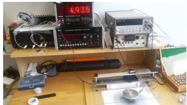
Figure 4 Experimental testing of the Hall-effect distance sensor
