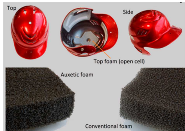
Figure 14 Application of auxetic foam in sports helmet [27]
