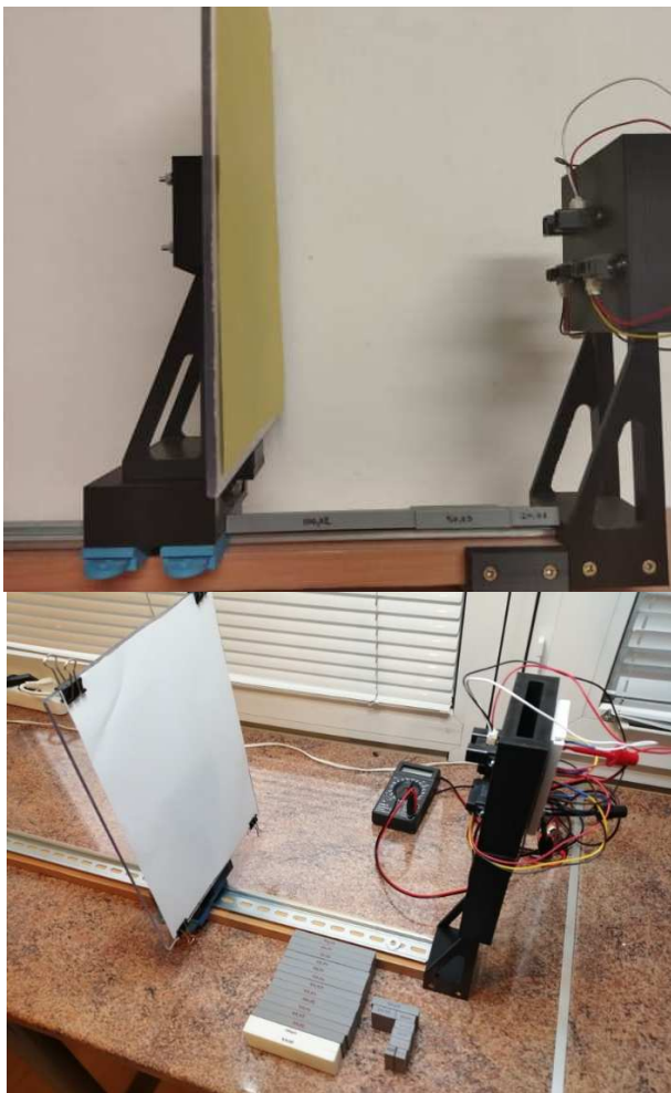
Figure 6 Improved apparatus for testing the optical distance sensor
