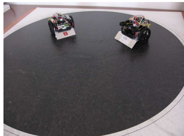
Figure 3 Sumo robots with applied optical distance sensors
