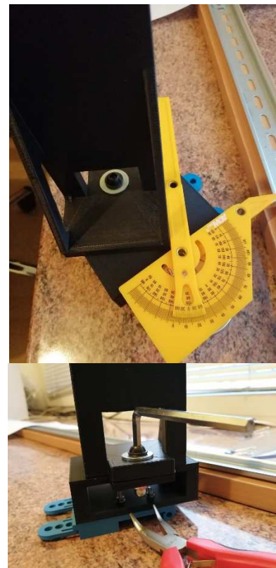
Figure 7 Adjusting the rotation of the reflective surface
