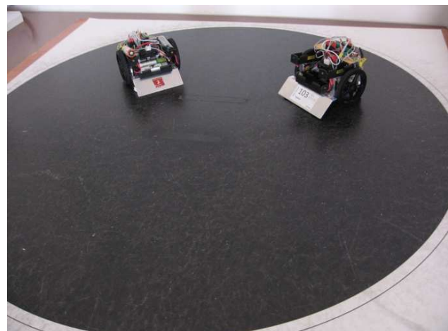
Figure 3 Sumo robots with applied optical distance sensors
