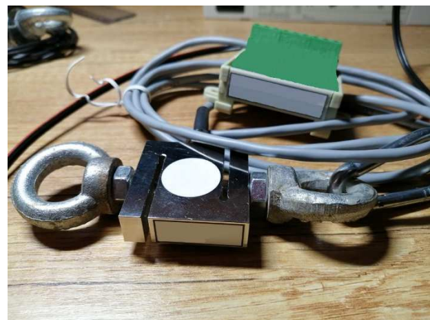
Figure 2 Measurement chain with force sensor
