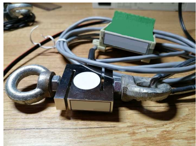
Figure 2 Measurement chain with force sensor
