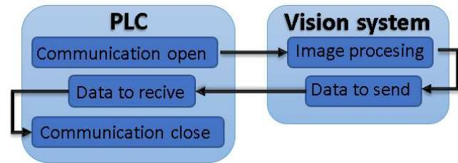
Figure 2 Principle of TCP / IP protocol communication
