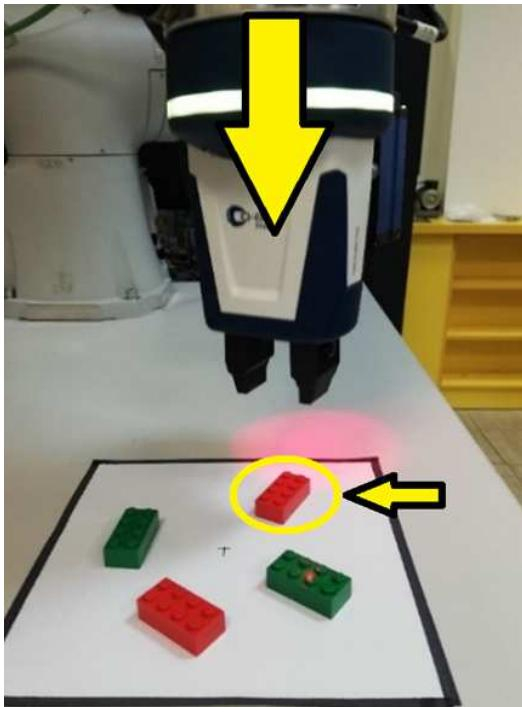
Figure 4 Pick & Place position for a founded object
