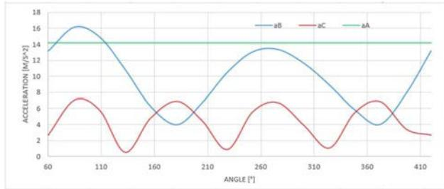
Figure 9 Acceleration of single points as a function of the angle of rotation of the member 2
