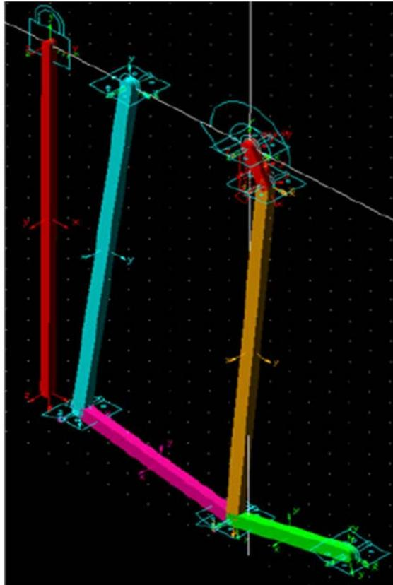
Figure 3 Kinematic model of the crusher mechanism
