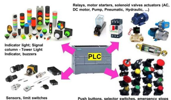
Figure 1 PLC in conjunction with sensors, actuators, controls and output modules
