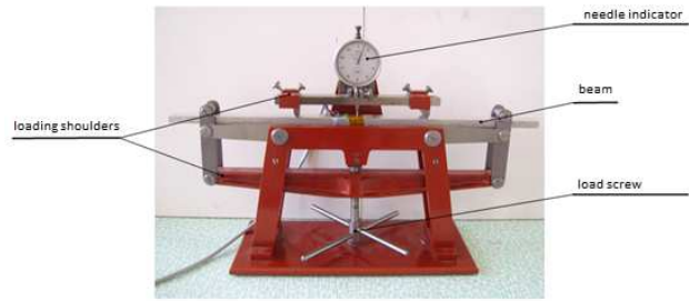
Figure 8 Beam clamped to the loading device
