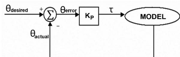
Figure 6 The control system with proportional feedback
