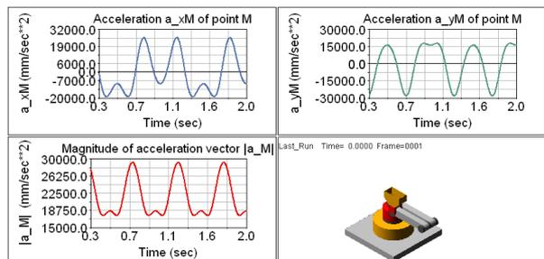
Figure 19 The graph of the acceleration  $a_{xM}$  and  $a_{yM}$  of the end-effector
