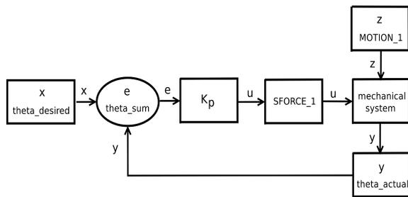
Figure 7 Scheme of control system with proportional controller
