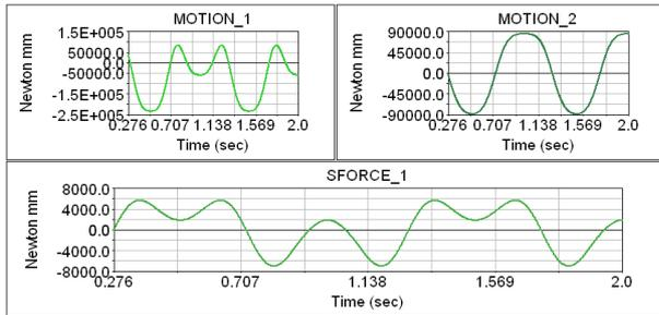
Figure 16 The graphs of the torques in the joints with weight of the basket  $m_b=10\text{kg}$
