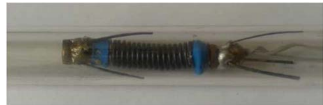
Figure 3 Machine with shape memory alloy actuator
