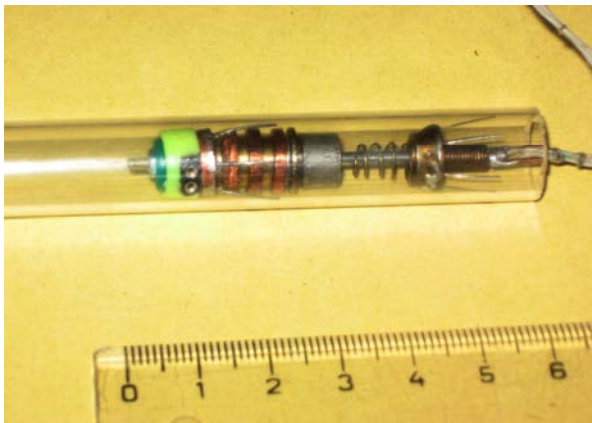
Figure 1 Machine with electromagnetic actuator
