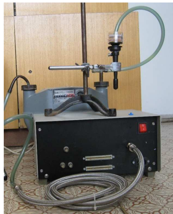
1 – dusty air, 2 – cyclone, 3 – filter, 4 – volume flowmeter, 5 – high-volume pump, 6 – analytic scales
