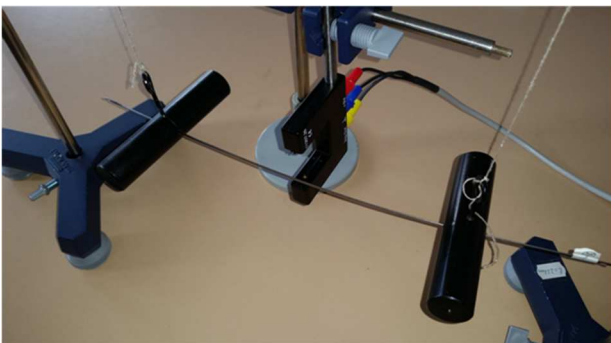
Figure 3 Experimental assembly. Vibrating wire sample crosses the infrared beam of an optical sensor (prismatic body with the shape of figure U in the centre of operation)
