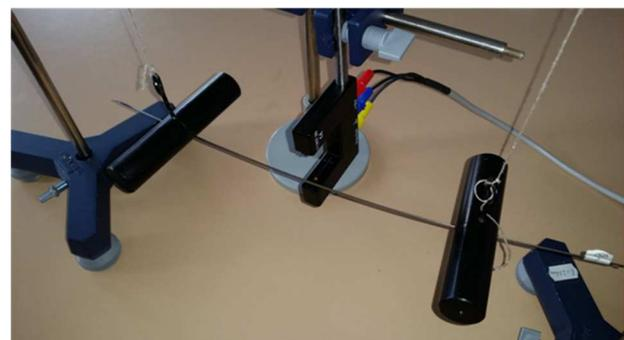
Figure 2 Experimental assembly in horizontal arrangement. Vibrating wire sample crosses the infrared beam of an optical
