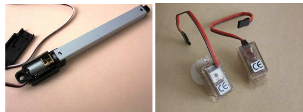
Figure 7 Rotational and linear RC servo
