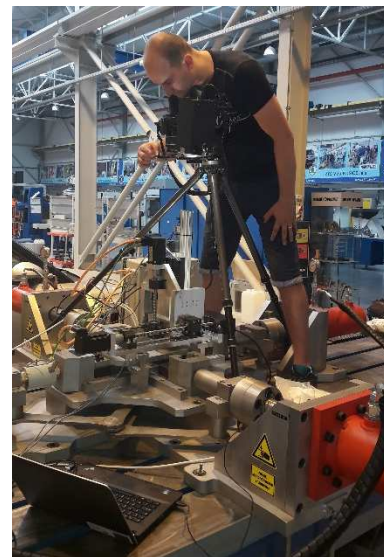
Figure 4 Drilling with positioning device and measuring of stresses with the optical device LF/Z-2
