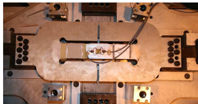
Figure 3 Aluminum sample with applied strain gauge cross
