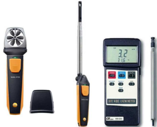
Figure 6 Vane anemometer and two hot wire anemometers
