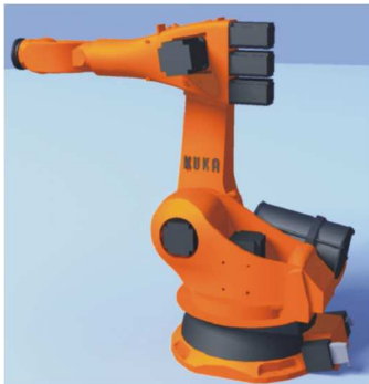
Figure 5 Mastering position – approximate position
